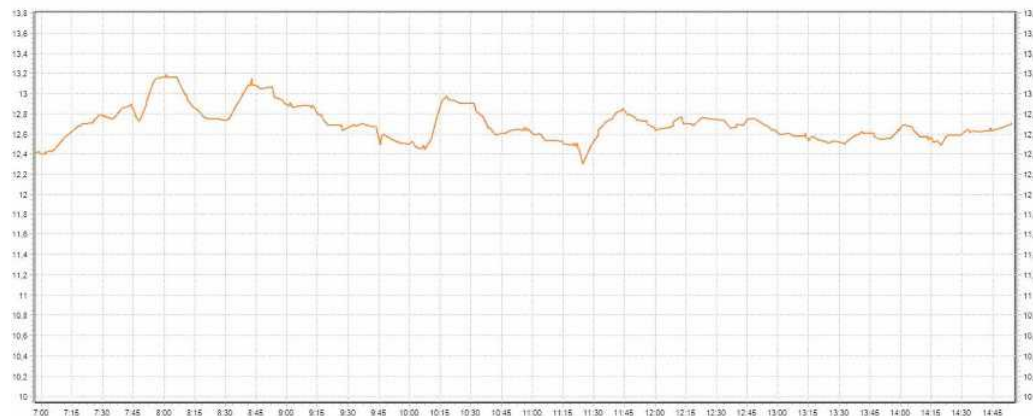
Figure 6: Example of a control chart showing TDS content in the pulp feed to a fiberline. This data is obtained by Vaisala Polaris PR53SD Process Refractometers.
